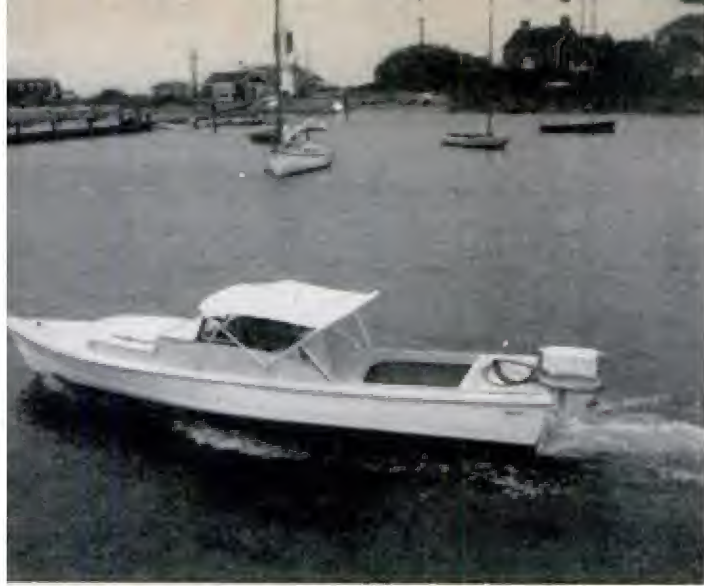
WHILE ACCELERATING , center of gravity remains forward, bow doesn't rear up, avoiding huge wakes
